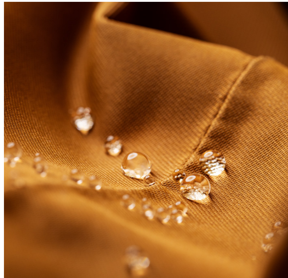
Water-repellent fabric in which PFAS is used to give dirt- and water-repellent properties.
